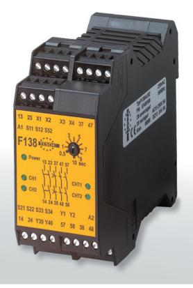
opening of the emergency stop contacts, or before switching on the power supply, the unit cannot enter into the "ready" state (i.e., it cannot be re-set). In auto-start mode (terminals X1-X2 and X3-X4 shorted), the unit becomes operational immediately upon the power supply being switched on, if the emergency stop, feedback, and re-set circuits are closed.
